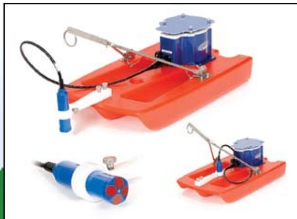
*The StreamPro's transducer can be towed from different points on board the platform, or can be removed and hand-held in the water for applications such as under ice flow measurements.*
